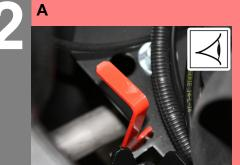
Engine is running but machine is not moving A Check setting of freewheel lever
