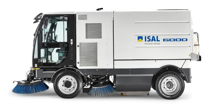
The combined **mechanical / suction / filtering** collection guarantees powerful and fast loading of any type of material from dust to leaves, as well as gravels ad large debris. An effective suction system optimises the collection of dust and light materials and the filtering system, made up of a battery of polyester filters, captures fine dust particles up to PM1 under all operating conditions, by eliminating almost completely the introduction of pollutants into the atmosphere.
